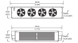
The D5 is a modular system consisting of an evaporator unit, D5-E, that is mounted at the back of the bus to the interior of the roof or on a structural attachment to the bus frame. The evaporator unit is connected to either an optional skirt-mounted condenser, D5-CS, or to an optional rooftop condenser, D5-CR. The supply air is distributed through ducts running on each side of the bus. Access to the fuse panel and circuit breakers is provided through a panel on the rear of the unit.
