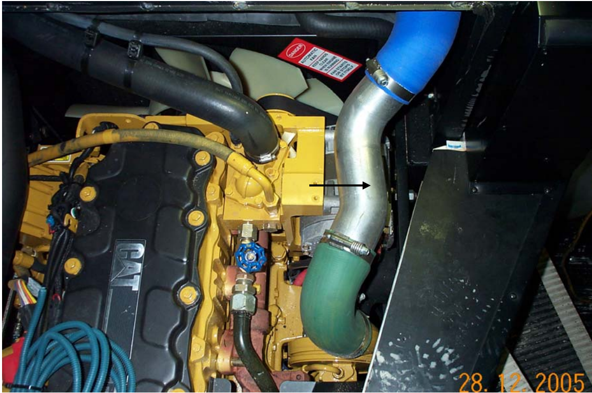
Turbo Tube may need to be rotated away to make room for P/S compressor.
