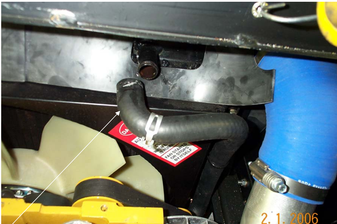
Trim Overflow Hose approx. 3/8" so it clears compressor pulleys. See next picture.
