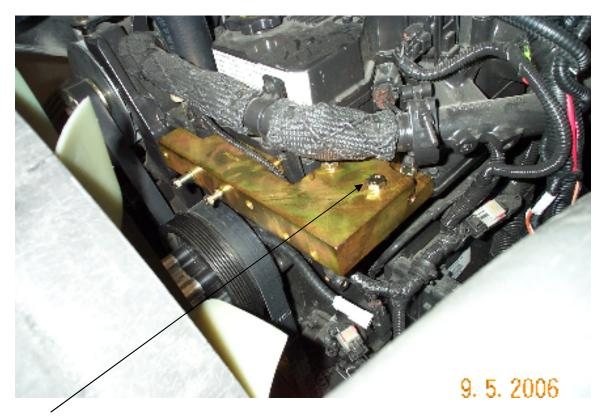
Install bolts finger tight to hold in place then put on Main Bracket
