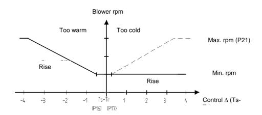
All the positions like (Px) are manipulated variables <Parameters>
