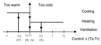
**Heating:** If the room temperature drops more than 0,5K below the set point temperature, the control switches on the heating. If the room temperature reaches the set point the heating is switched off.
