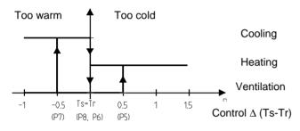
**Heating:** If the room temperature drops more than 0,5K below the set point temperature, the control switches on the heating. If the room temperature reaches the set point the heating is switched off.
