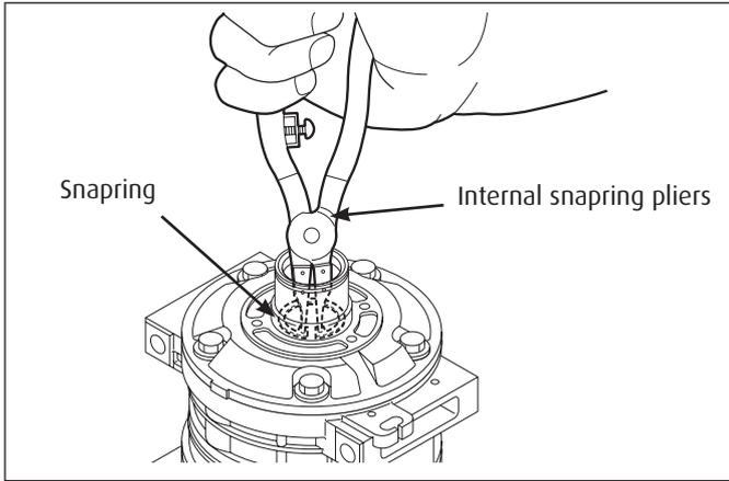
6. Install the snap ring using internal snap ring pliers. Press the snap ring using the installing end of the remover (597035-5520) until a "click" is heard.
