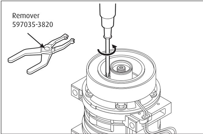
5. Remove the field coil's lead wire bushing using the remover (597035-3820).
