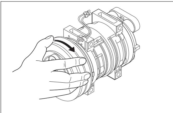
3. When installing the compressor in service system, the compressor should be installed after adjusting the amount of oil, referring to "oil check" p.16.
