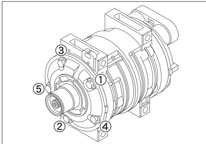
8. Mount the new gaskets on the through-bolts. Insert the five through-bolts from the front cylinder head side and tighten them to the specified torque. Each bolt should be gradually tightened in three or more stages to ensure the specified torque.
