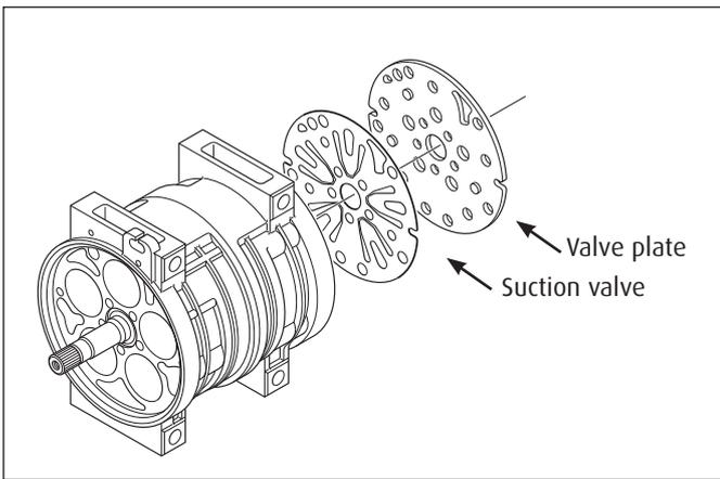
9. Remove the valve plate and suction valve from cylinder shaft assembly, then remove all the gasket material from the valve plate.
