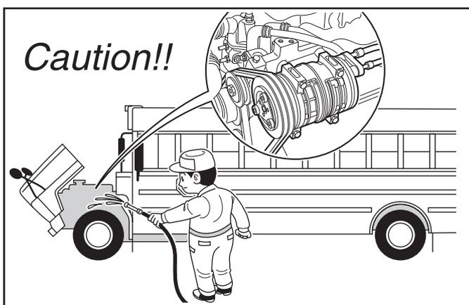
4. Keep the compressor clear of water projection while cleaning the vehicle.
