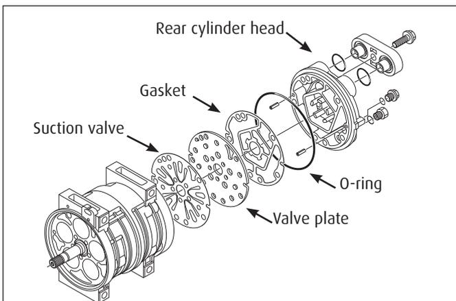
5. Coat the new O-ring with clean compressor oil and install it on the rear cylinder head.
