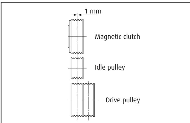
2. Ratio of magnetic clutch to drive pulley
