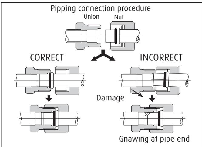
3. Fit the nuts and unions tightly against the base of the companion pieces, then hand tighten the nut as much as possible. Then tighten to the specified torque.
