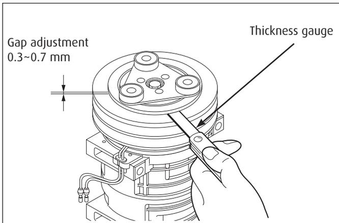
7. Check that the clutch clearance is as specified. If necessary adjust the clearance using shim(s). Adjusting shims are available in the following thickness:
