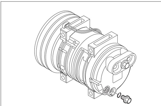
9. Install the oil drain plug with a new O-ring, thinly coated with clean compressor oil, and tighten it to the specified torque.
