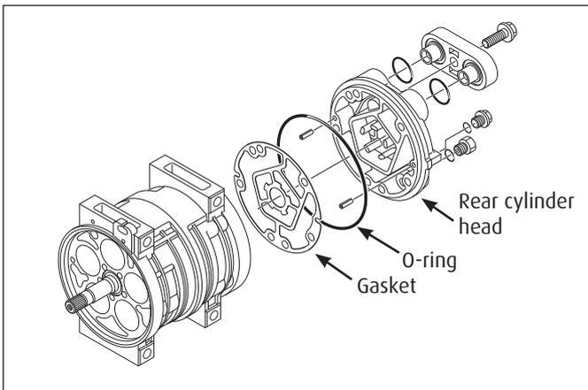
8. Remove the O-ring from the rear cylinder head, and then remove all the gasket material from the rear cylinder.
