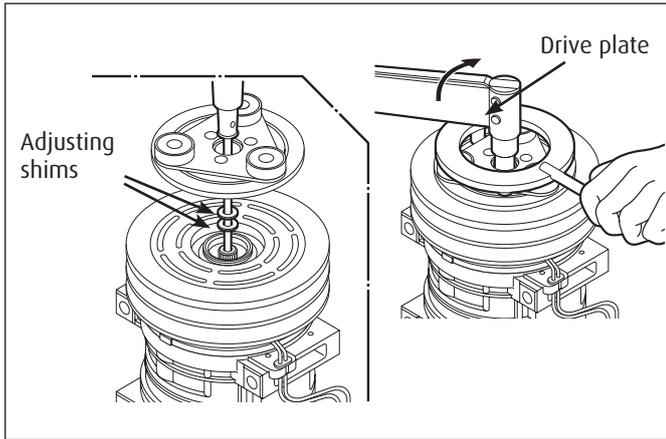
5. Install the armature assembly on the driveshaft together with the original shim(s). Press the armature assembly down by hand.
