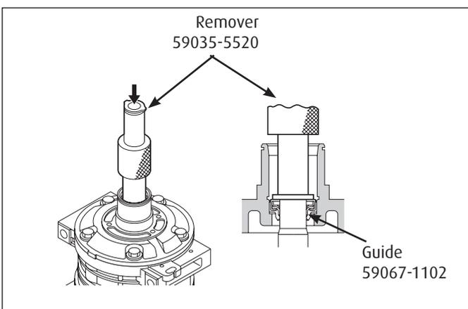
5. Install the shaft seal as far as possible into the front cylinder head using the installing end of the remover (597035-5520). Remove the guide (597067-1102) from the drive shaft.
