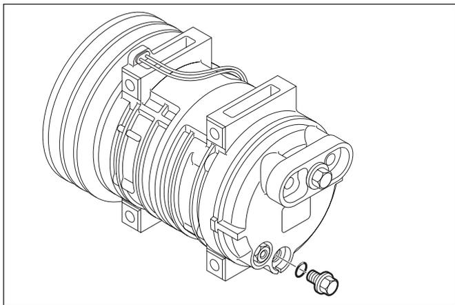
Install the oil drain plug with a new O-ring, thinly coated with clean compressor oil, and tighten it to the specified torque.
