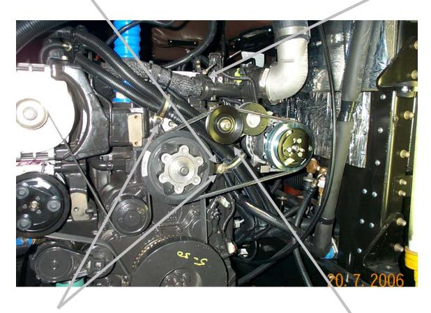
Main Power Conductors have to be secured firmly to engine so that tensioner does not hit them.
