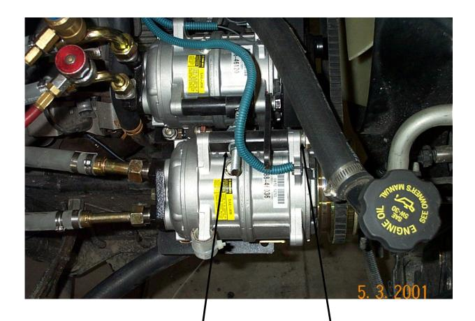
Tension outer compressor with this nut
