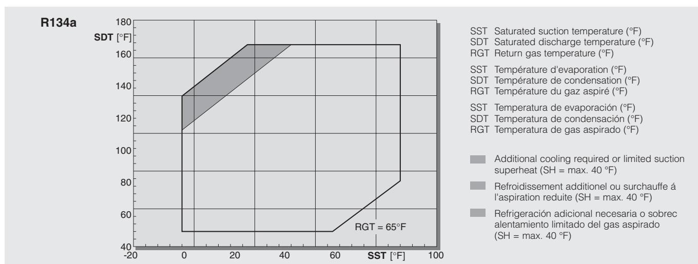
When using a capacity control, the application limits may shift.
